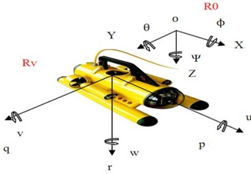
Fig. 1. Body-fixed frame and earth-fixed reference frame for the SUBSEA-TECH ROV.
