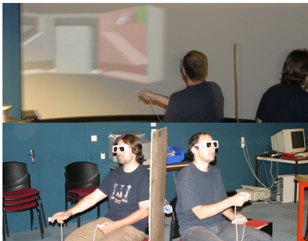
Figure 6: snapshots of the experimental setup. Each user holds 2 input devices: one 3D tracker (dominant hand) and one "trigger" device with buttons (non-dominant hand)
