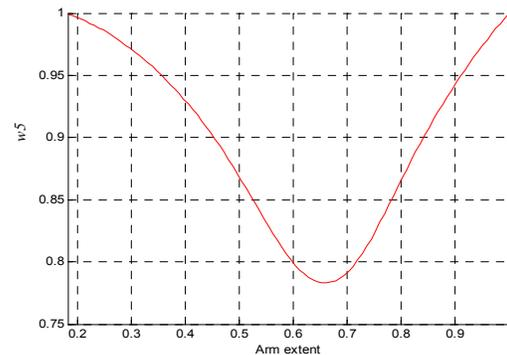
Figure 3. Arm Manus manipulability for positioning task
