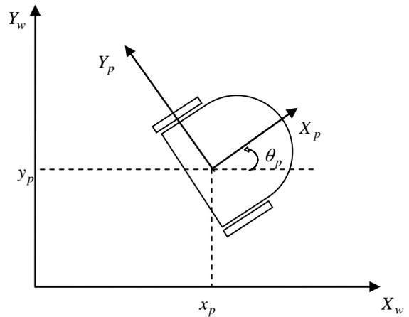
Figure 2. Wheeled mobile platform
